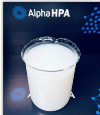
Sol-gel formation from high dispersible boehmite
