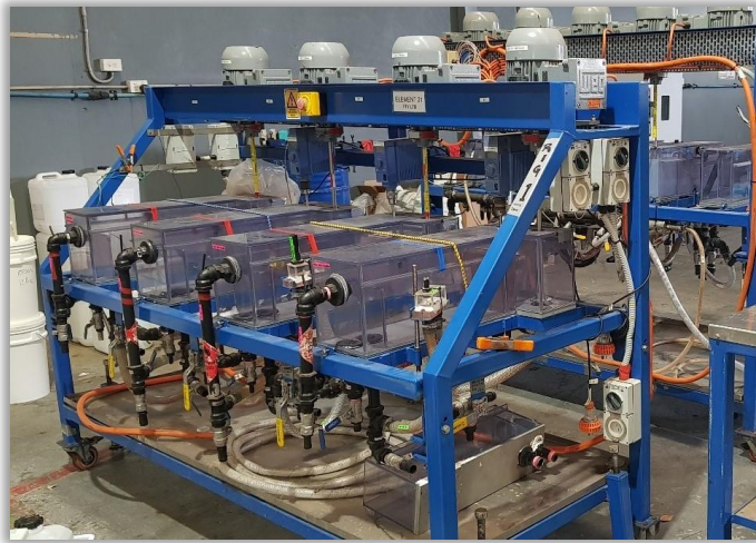
Solvent Extraction (SX) Pilot Rig
