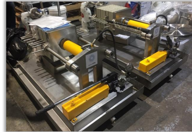
Pilot Plant Filter Presses
