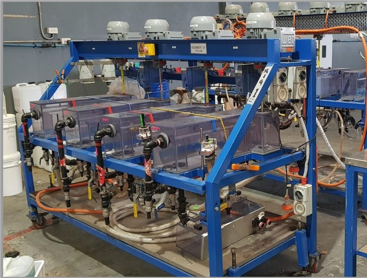
Solvent Extraction Pilot Rig
