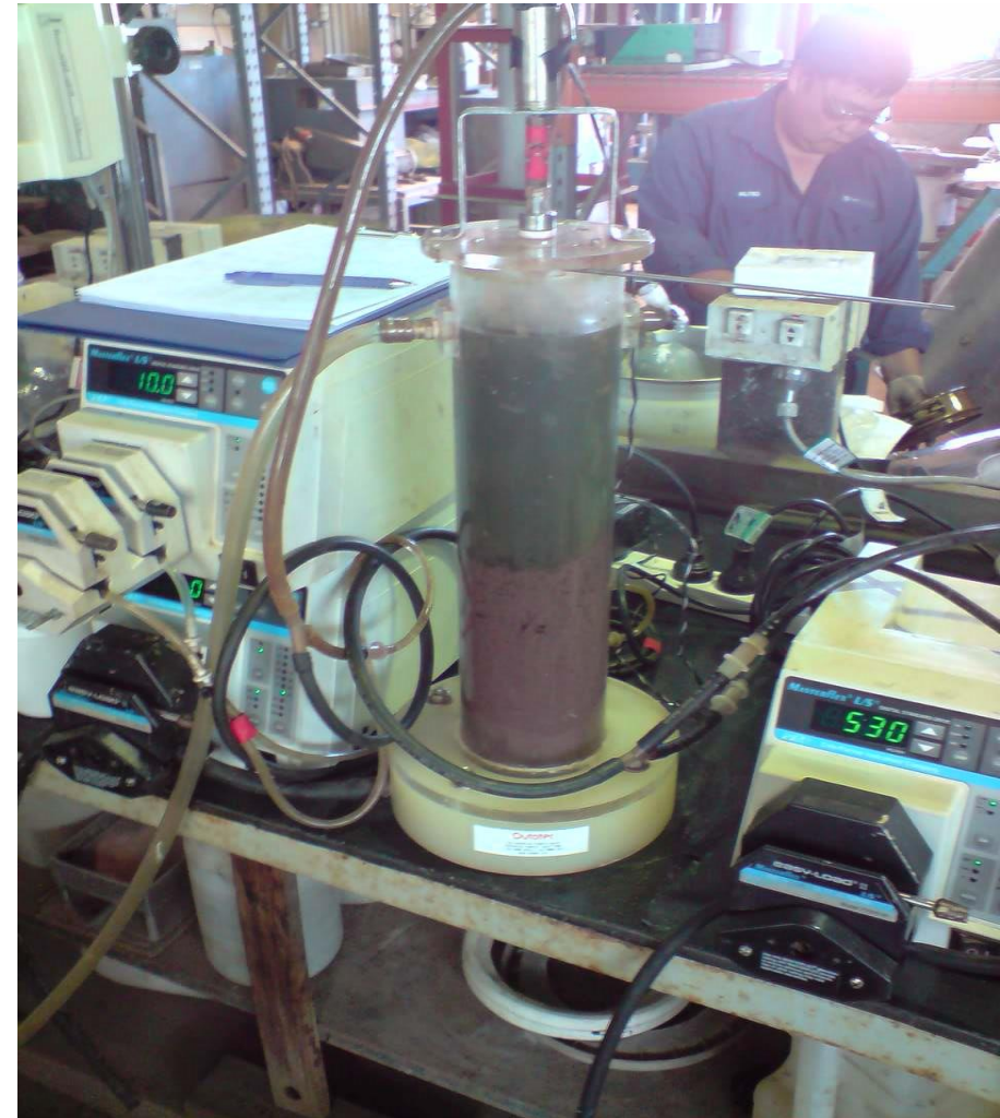
Settling test on CCAL discharge slurry (separation of residue solids from pregnant solution).
