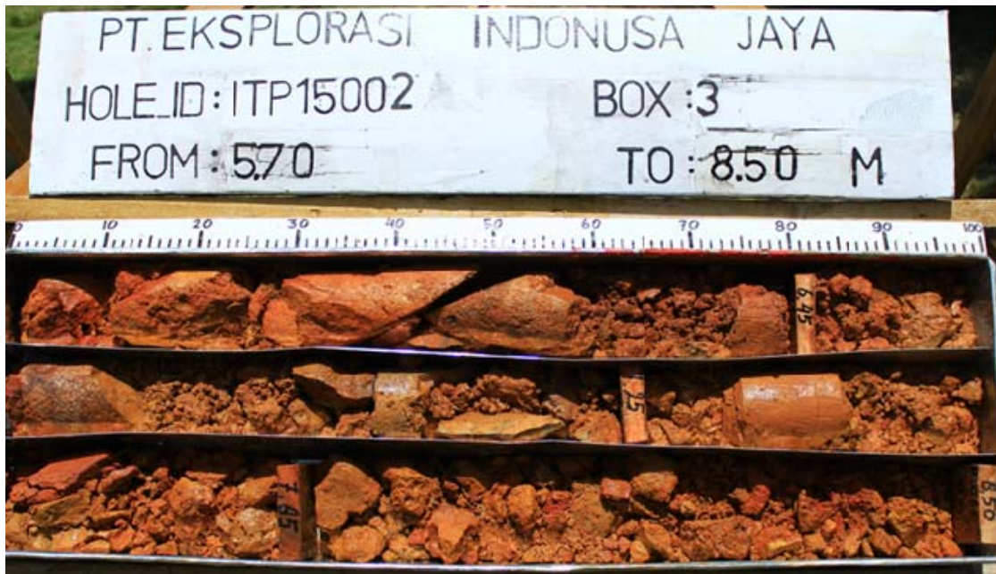
Drill core from Tapadaa drill hole ITP15002. Intensely oxidised vuggy quartz grading 0.63 g/t gold over the interval 5.0 to 9.0 metres is shown.
