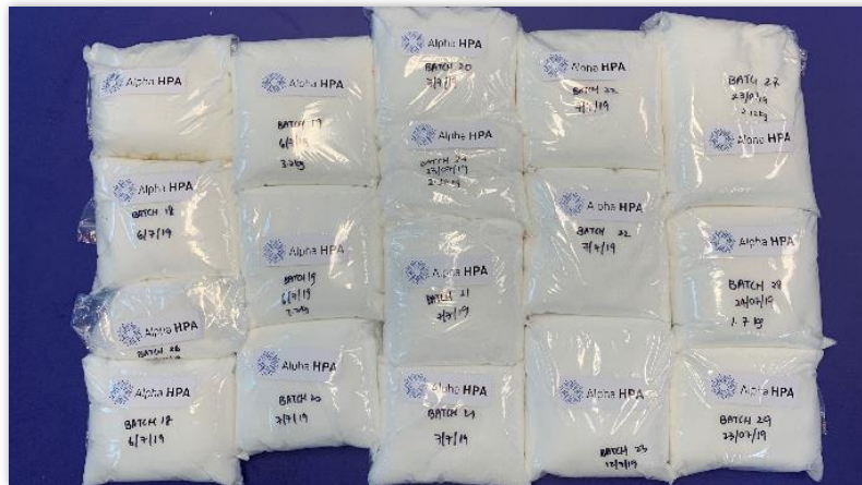
Figure 10: 21kg of high-purity aluminium salt, generated in the Pilot Plant over a 24 hour period
