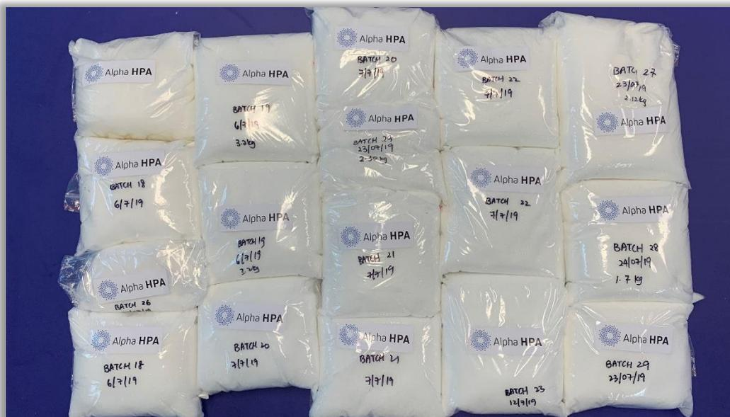
Approximately 21kg of high purity (>99.99%) aluminium salt generated over a 24-hour operating period
