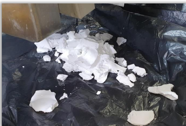
HPA pre-cursor generated from filter commissioning
